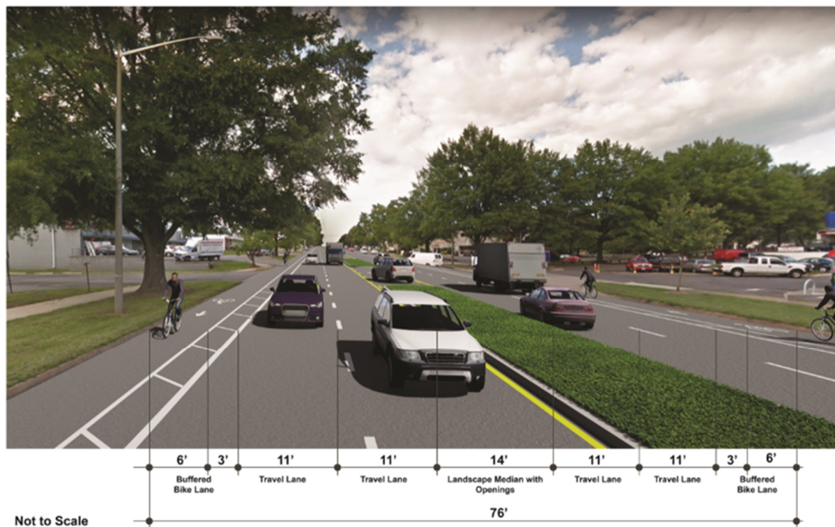
Exhibit 1. Cross-Section Concept with Landscaped Medians with Openings and Buffered Bike Lanes
